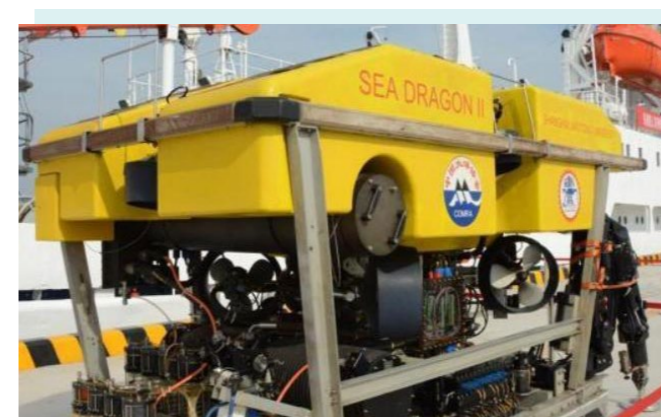
圖 2：無人遙控潛水器 Picture 2: Remotely Operated Vehicle (ROV)
